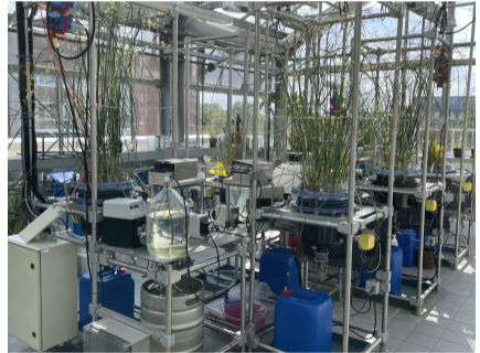
Figure: Planted Fixed Bed Reactor
